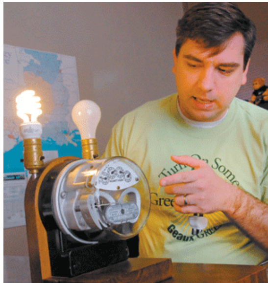
Energy Corp. spokesman Philip Allison uses a power meter to demonstrate the amount of energy a compact fluorescent light bulb uses compared with a standard light bulb. (Photo by Frank Aymami)
